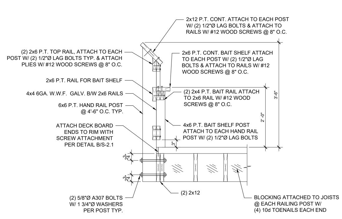
C FISHING RAIL DETAIL AT PIER ENDS SCALE: 1"=1'-0"
