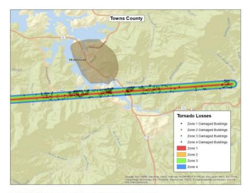
Figure 12: Modeled EF3 Tornado Damage Buffers in Towns County
